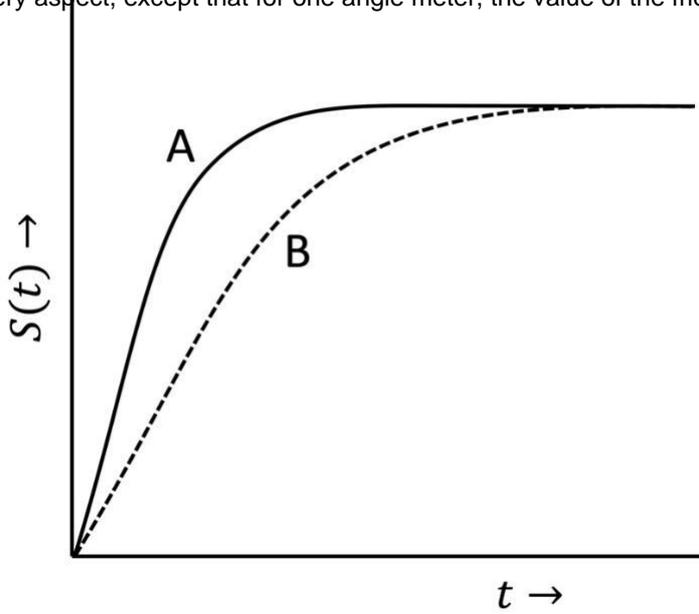
Figure 2.3 Step responses of two different angle meters, A and B.
