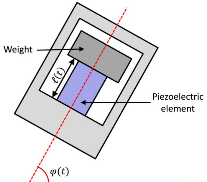
Figure 2.2 Inside of the angle meter
