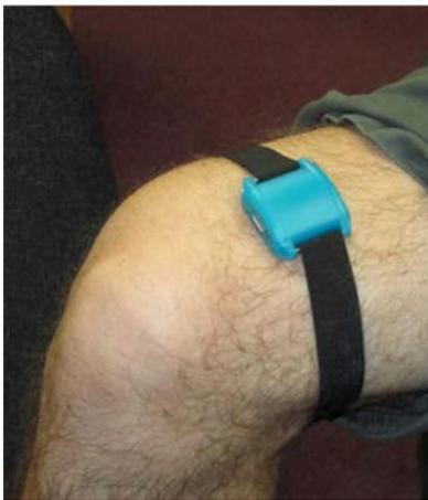
Figure 2.1. Angle meter attached to the upper leg.
